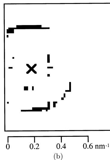
Fig. 6. SANS patterns from sample A, (a) 100 peak, (b) 001 peak. A threshold has been used to reveal the slight anisotropy present in the two primary diffraction rings. The X marks the position of the unscattered beam.
